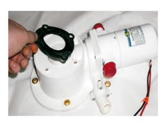
10. Remove the inlet and outlet protection covers of the new kit.
